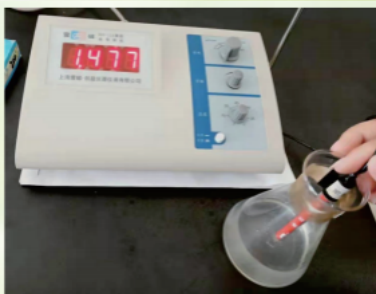
Initial conductivity measurement for hydroponic experiment in Xinjiang: 1.477 mS/cm
